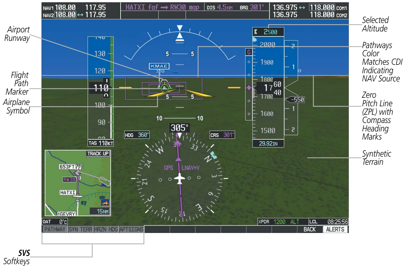
Figure 8-3 SVS on the Primary Flight Display
